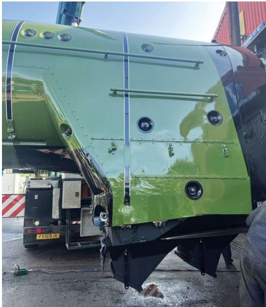
Above: ...and while still suspended the ashpan was fitted.
