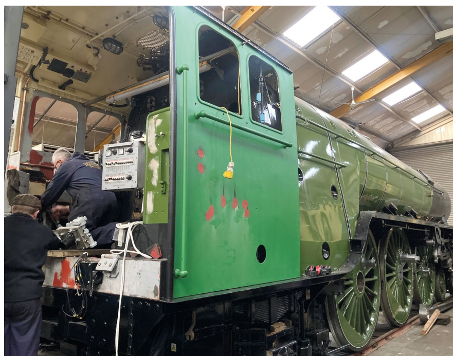
Above: The cab back on the frames and work already underway to test the ETCS equipment.
