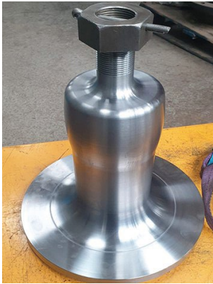
The newly machined bogie pintle.
