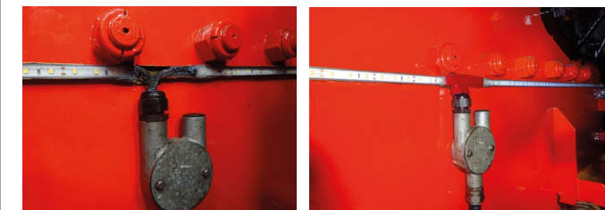
Above left: Exposed wiring connections to driver's side front inside LED lighting strip and right, a new protective cover over wiring connections to driver's side front inside LED lighting strip.
