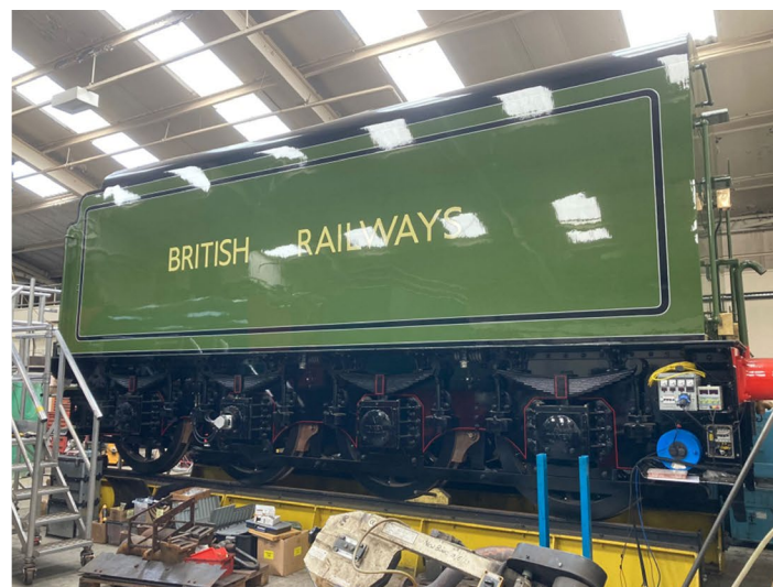
Above: The cab back on the frames and work already underway to test the ETCS equipment.
