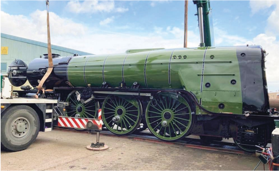
Right: The locomotive's frames were then run out and the boiler carefully lowered.
