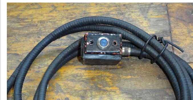
Existing sander indicator LED box (to be refurbished and reused).
