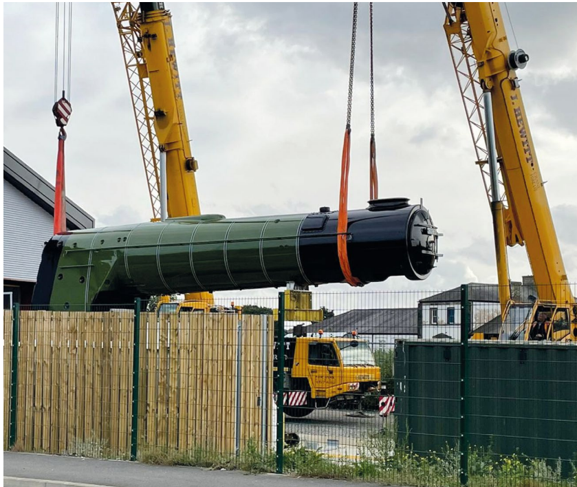
Above: ...and while still suspended the ashpan was fitted.
