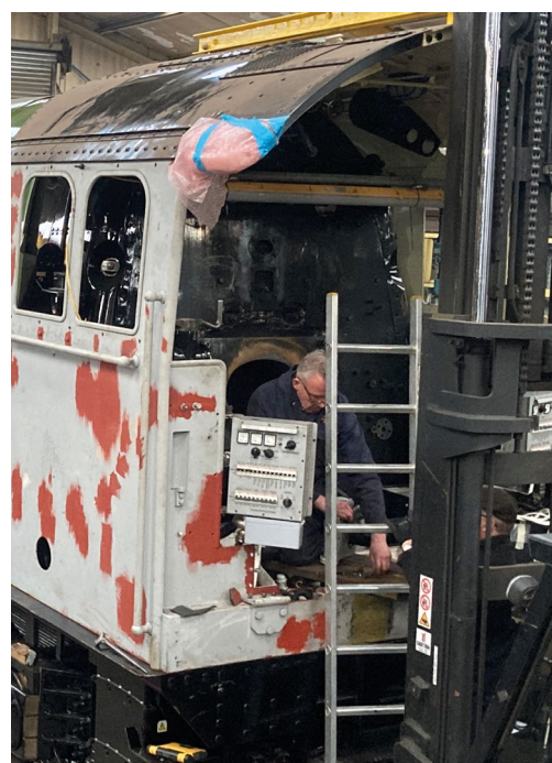
Above: The cab back on the frames and work already underway to test the ETCS equipment.
