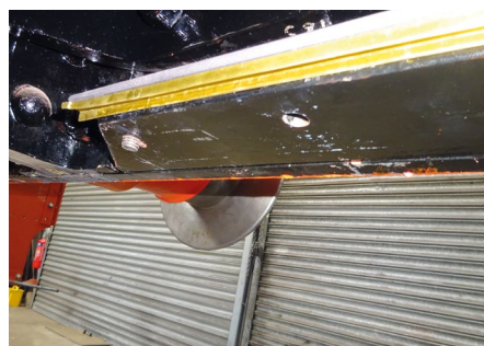
Above images: New front buffer beam LED lighting strip trough in place behind the buffer beam.
