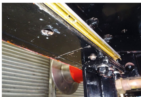
Above images: New front buffer beam LED lighting strip trough in place behind the buffer beam.
